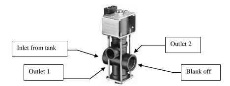
Connect the solenoid cable from the control box to the outlet cable on the solenoid. With electrical power to the solenoid off, flow to outlet 1 is stopped, and foam flows to outlet 2. With electrical power to the solenoid on, flow to outlet 2 is stopped, and foam flows to outlet 1.
